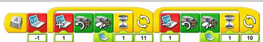
This program starts the fan from rest, accelerates it to a power level of 10, and then decelerates back to rest.
