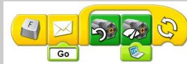
When “F” is pushed, a message is sent to each loop. The tilt sensor determines the value of the display which also determines the speed of the motor.
