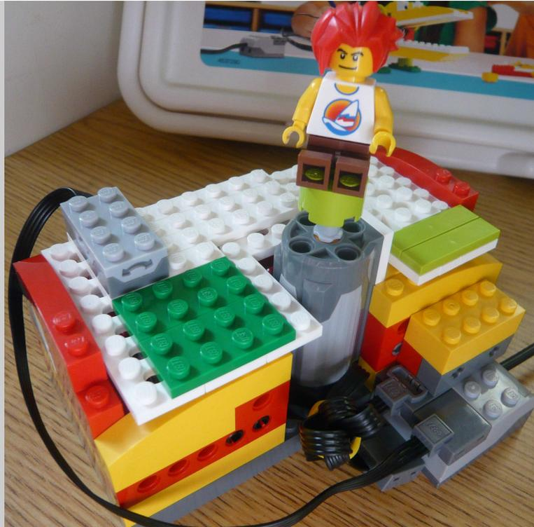
1. Begin with a class discussion about programming and sensors. Explain the difference between the tilt and motion sensors. The tilt sensor can be used to determine the orientation or position of the music box lid. The motion sensor can be used to determine how far open the music box lid is from where it started.
