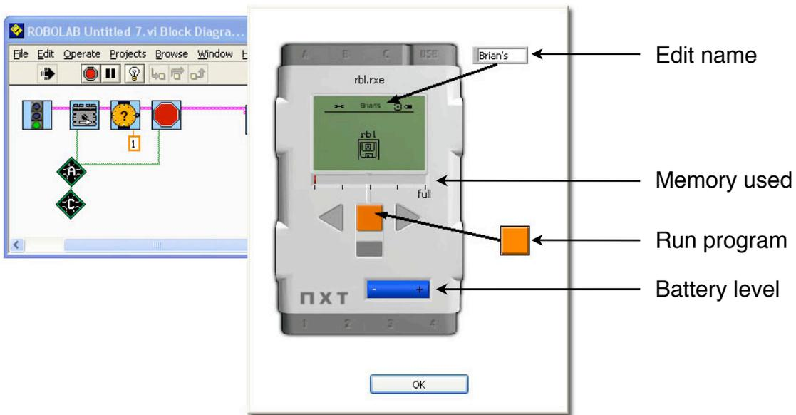
Note - the very first time you talk to the NXT (or RCX), ROBOLAB will download new firmware into the brick. On the NXT, this is fast and will remain in memory with or without batteries. The RCX will lose the firmware if it loses the batteries (like before).
